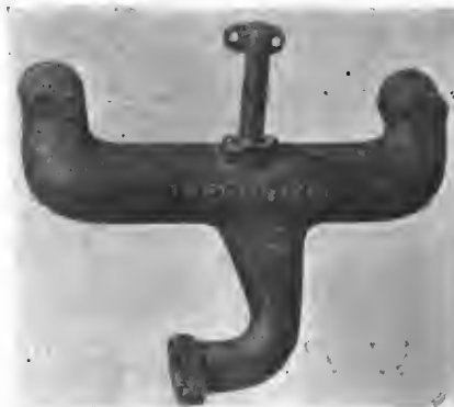
Thermo-Kor manifold for Fords, which heats the incoming mixture
